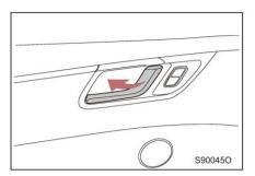
The door can be opened by pulling the interior door release handle.
