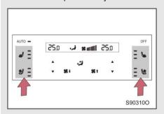
Touch the seat heating and ventilation buttons on the rear A/C operation panel to select the appropriate heating and ventilation gears.
