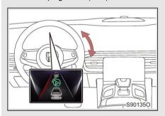
When the system determines that the vehicle has deviated from the lane, the corresponding side line turns red and flashes and a warning is issued, then the steering wheel corrects it automatically.
