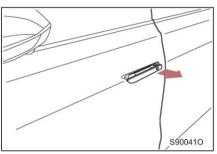
When the vehicle is locked, touch the door handle sensor switch to unlock the door and the door handle will pop out.
