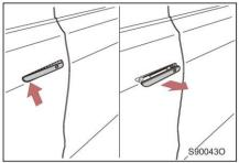
Press the front part of the driver side door handle to tilt it, then pull the middle part and pull it out vertically.
