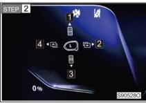
Operate the scroll wheel on the left side of the steering wheel and the left/right selection buttons to adjust the exterior rearview mirror at the corresponding side.
