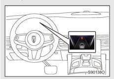
When the system determines that a collision may occur, the alarm information will appear on the instrument cluster and an alarm sound will be issued
