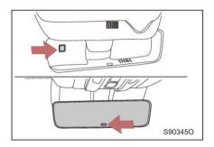
The interior rearview mirror is provided with automatic anti-glare function. It detects the ambient light intensity and the light intensity of the following vehicle through the front and rear light sensors, and the lens can automatically reduce the reflection when the light from the following vehicle is too bright at night.
