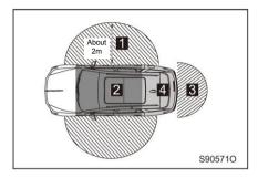
Effective range of the key sensing antenna: hemispherical area centered on the sensing antenna
