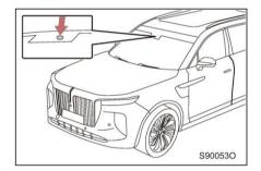
The light and rain sensor determines the amount of rain.
