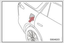
Method 1: When the vehicle is locked and the power (ignition) switch is set to OFF mode, carry your smart key with you, press the front end of the charging port cover, and it will open automatically; when the vehicle is unlocked, press the front end of the charging port cover, and it will open automatically.
