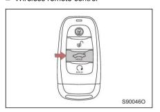
When the trunk lid is open, press and hold the button until the trunk lid is closed.
