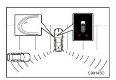
When the shift lever is in the R and the vehicle speed is 0-15 km/h, if there are crossing vehicles, electromobiles, bicycles and other targets in the lateral direction behind the vehicle, the system will judge whether there is a collision risk and the collision risk level of the relevant target. If any, the indicator in the corresponding side rearmirror lights up, and the multimedia system display shows an alarm message to avoid the collision.
