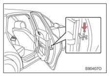
Disengage the mechanical locking switch guard of the corresponding side door.
