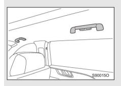
The ceiling handle is located at the roof side member of each door.
