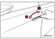
Hold the door handle, and lock and unlock the door with a mechanical key.
