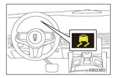
If the vehicle skids or the drive wheels are idling, the indicator flashes, indicating that TCS/ESC is operating.
