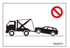
Do not tow with a lifting load trailer to prevent damage to the body.
