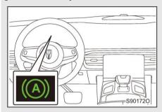
When the AUTO HOLD is activated, the AUTO HOLD indicator lights up on the instrument cluster.
