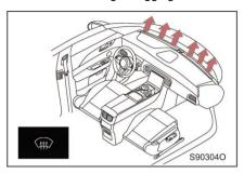
Touch the 'ss' button, the indicator will light up, and the forced defrosting/defogging of the front windshield will be activated.
