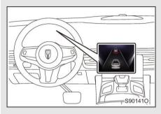
If the AEB is activated, the alarm information will appear on the instrument cluster and an alarm sound will be issued.
