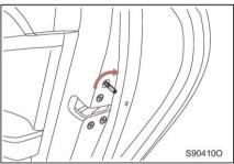
Use the mechanical key to close the doors after locking.
