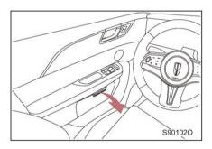
Storage boxes are located on each door. Pull the storage box cover to open the storage box.
