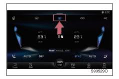
Touch the wbutton on the display, and the indicator will light up to start heating the rear windshield and exterior rearview mirror.
