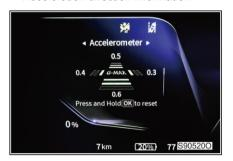
It displays the acceleration information of the vehicle in all directions.
