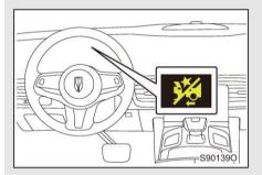
When the system is turned off, the instrument cluster will show FCW OFF indicator.
