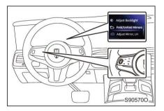
Operate the menu button on the left side of the steering wheel to enter the setting interface of backlight brightness and exterior rearview mirror, and select the exterior rearview mirror to fold through the scroll wheel on the left side of the steering wheel.
