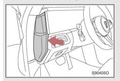
Detach the left cover plate from the instrument panel.
