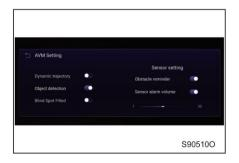
You can set the radar alarm volume and the automatic radar in the AVM interface of the multimedia system.
