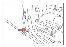
The manufacturer's nameplate is located on the right side B-pillar as shown in the figure.
