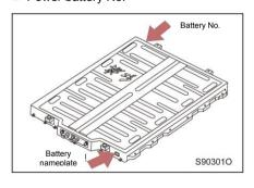
As shown in the figure, the battery No. and battery nameplate are located on the battery case body.
