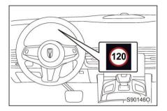
When the system recognizes the speed limit sign, if the vehicle speed is less than the speed limit value, the instrument cluster will only display the current speed limit requirement through the indicator; and if the vehicle speed is more than the speed limit value, the instrument cluster will remind the driver by sound/icon/text message, etc.
