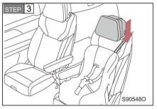
Fix the hook firmly to the anchor support and fasten the top strap.
