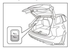
Close all doors, apply EPB, open the trunk lid and press the AirS lowering button to enter the loading mode.
