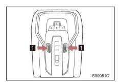
Touch the front reading lamp button to turn on the lamp, and touch the button again to turn off the lamp.
