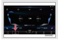
When the vehicle speed is less than 15 km/h, press the PDC/RVC ON/OFF button, and it will light up, which indicates that the PDC is turned on; press the PDC/RVC ON/OFF button again, and it will go out, which indicates that the PDC is turned off.
