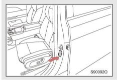
A tire pressure label is attached under the driver's side B-pillar locking pin.
