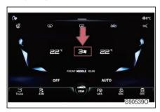
Method 1: slide up/down the air volume setting value in the operation display of A/C to adjust the air volume of the A/C system among level 1-7.
