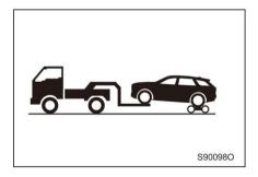
Place the towing trolley under the rear wheels and put the vehicle into lift mode.
