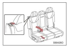
For seven-seat models, if you want to access the third-row seat, you need to pull the shoulder adjustment handle of the second-row right seat, fold the backrest to the 45° position and move the right seat forward.
