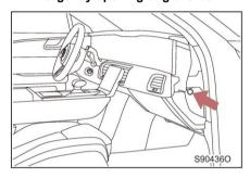
When the glove box cannot be opened normally through the glove box switch, emergency opening is available through the glove box cable.
