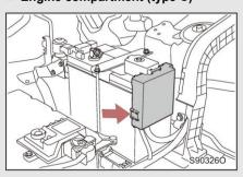
Press the retaining clip to open the cover.
