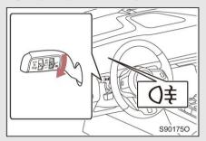
Toggle the fog lamp switch down to turn on the rear fog lamp, toggle the switch again to turn off the rear fog lamp
