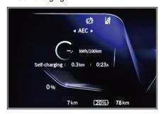
It displays the average energy consumption/mileage/running time of the vehicle after self-charging.
