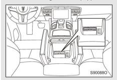
The back of cell phones that support Qi standard wireless charging can be placed directly in the wireless charging area for charging.
