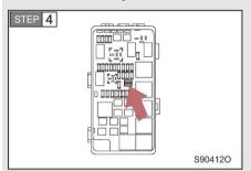
Remove the fuse with the remover.
