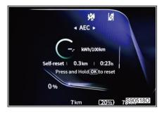
It displays the average energy consumption/mileage/running time of the vehicle after resetting.
