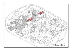
When the vehicle is in some serious front impact, the pretensioner will activate, tighten the seat belt, and quickly restrain the occupant to better protect the occupants.
