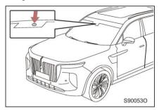
If an object is placed on the sensor or if there is an attachment on the windshield that obscures the sensor, the sensor may not be working properly.
