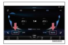
Touch the [AUTO] button, the working indicator lights up and enters the automatic air conditioning mode.
