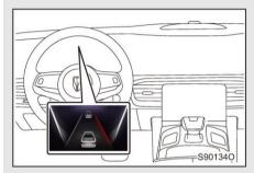
When the system determines that the vehicle has deviated from the lane, the corresponding side line turns red and flashes and a warning is issued.
