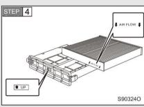
Detach the filter from the filter housing and replace it with a new one.
