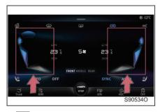
Touch the air outlet mode button to select the corresponding air outlet mode, and touch the button again to cancel the air outlet mode. The air outlet mode can be selected in combination.
