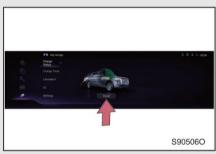
Method 2: Touch the charging port cover switch in the charging settings of the multimedia system, and the charging port cover will open automatically.
