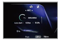
It displays the average energy consumption/mileage/running time of the vehicle after start.
