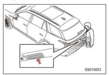
When the vehicle is locked, if you carry the smart key, you can press the external opening button of the trunk lid to unlock and open the trunk lid; when the vehicle is unlocked, press the external opening button of the trunk lid to unlock and open the trunk lid.
