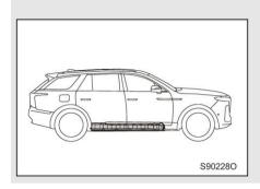
The power battery is arranged under the vehicle floor.
