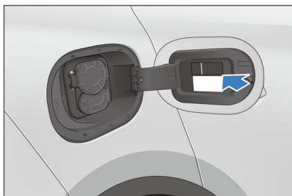
The charging indicator label is attached to the inner side of the charge port hinge.
